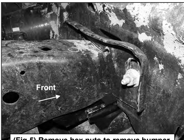
(Fig 5) Remove hex nuts to remove bumper
