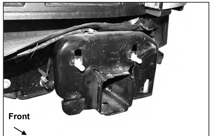
(Fig 6A) Remove factory double bolt plate
