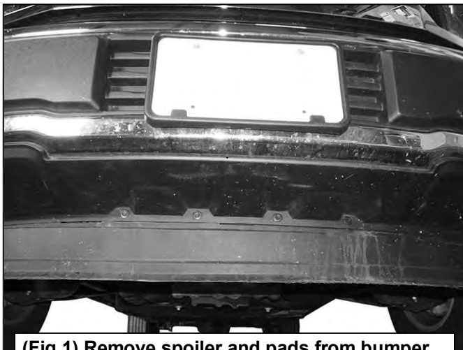
(Fig 1) Remove spoiler and pads from bumper
