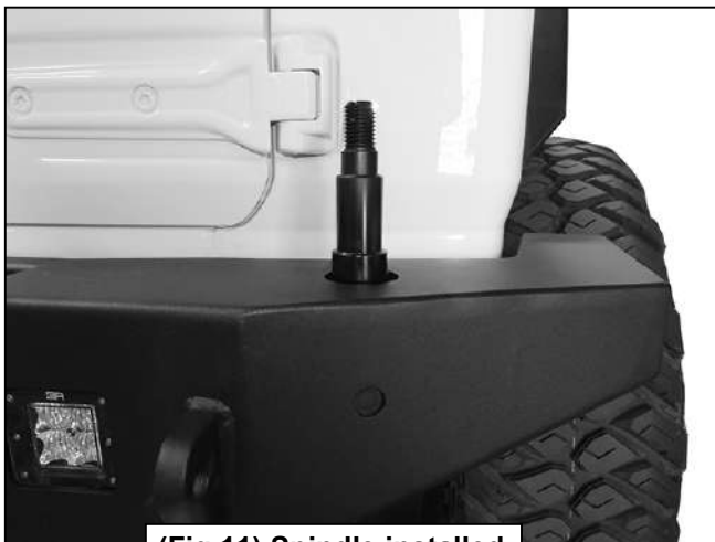
(Fig 11) Spindle installed
