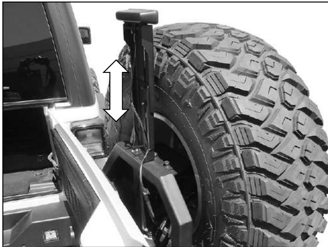
(Fig 29) Swing Arm assembly installed
