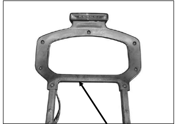
(Fig 26) Remove cover from factory light bracket
