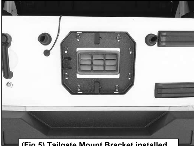
(Fig 5) Tailgate Mount Bracket installed
