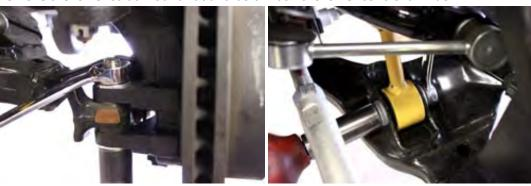
5. Remove the three upper strut mounting bolts. Remove the strut from the vehicle and mount it in a vise. Install the Maxtrac leveling kit, and torque fasteners to OEM specs.
