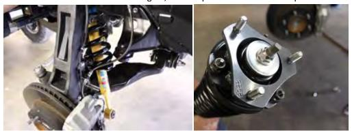
6. Reinstall the strut assembly. Leave the three upper strut mounting nuts loose. Raise the lower control arm and install the lower strut mounting bolt and nut. Use a floor jack to raise the lower arm up in order to get the lower ball joint bolts installed. Be sure to use thread locker on the lower ball joint bolts. Tighten all bolts to factory spec.
