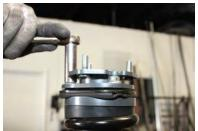
8) RE-INSTALL THE STRUT BACK INTO THE TRUCK USING PROVIDED NUTS ON TOP AND THE FACTORY BOLT ON THE BOTTOM, THEN ADJUST THE JACK UP SO THAT THE LOWER CONTROL ARM CAMS CAN BE RE-INSTALLED. ONCE INSTALLED, LINE UP YOUR MARKS AND TIGHTEN THE CAM BOLTS.
