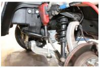
**3)** REMOVE THE LOWER STRUT BOLT THEN REMOVE ALL THREE NUTS AT THE TOP OF THE STRUT.
