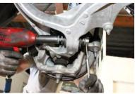
**4)** SUPPORT THE LOWER ARM WITH AN ADJUSTABLE JACK, MARK A REFERENCE LINE ON BOTH LOWER CONTROL ARM CAM BOLTS, THEN LOOSEN AND REMOVE BOTH BOLTS.
