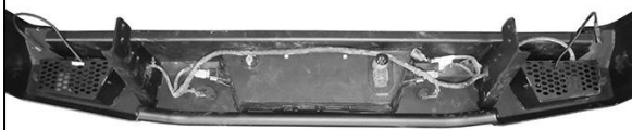
(Fig 7) Attach sensors and wiring harness to Bumper as equipped. Plug Harness Extensions into outer plugs in harness
