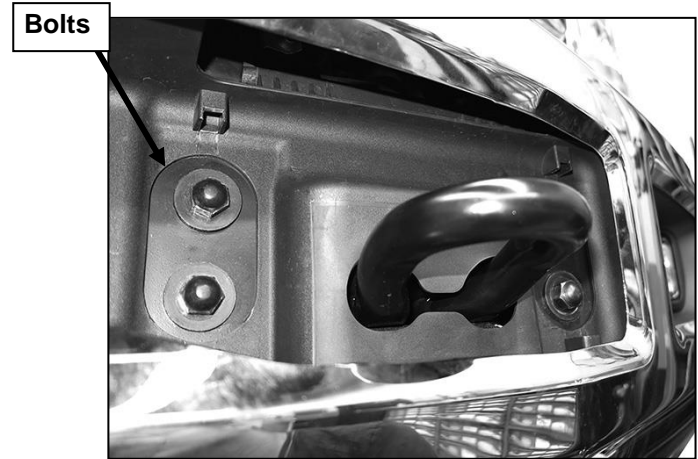
(Fig 6) Remove bumper bolts (driver side pictured)
