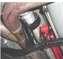
OPTIONAL WELD-IN DRIVESHAFT LOOP INSTALLATION: Remove one end of the driveshaft and slide the driveshaft loop over it. Reinstall driveshaft. Position the loop 6 inches from the front u-joint. Mock it up so that there is sufficient clearance to allow the driveshaft to go up and down 1.5". Using the provided length of tubing, cut and weld the ends to allow mounting the loop to the crossbrace. Double check the clearances and weld into place.
