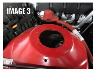
5. Remove the brace and de-burr the mounting holes.
