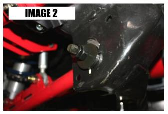
main nut and rotate the camber bolt to the desired setting using a 12mm Allen wrench.
