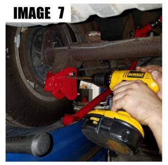
16. Insert a 1/2" x 1.25" bolt, washer, and nut and tighten with a 3/4" wrench and socket.
