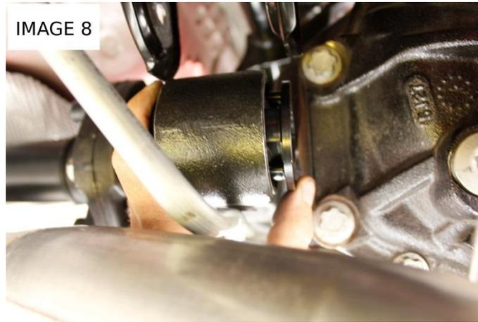
11. Position large rear bushing lockout, with the smaller counterbore facing the rear of the vehicle, into the rear bushing housing and tap in with a hammer. Existing bushing removal or modification is not necessary. This one is tricky, as the bushing housing is usually oblong. It is usually easiest to tap one side of the lockout in, then tap the other. Excessive force to seat this is not necessary. If a gap exists, it can be further seated by torquing the large bolt down to spec. **IMAGE 9**
