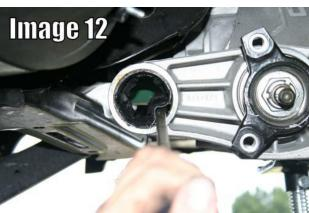
14. Place some rags between the inner CV boots and the cradle to protect the boot then lower the differential to gain access to the front
