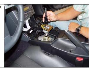
**STEP 12.** File out approx. .125" from shifter casting in indicated area. Clean out metal chips and relube entire pocket with provided grease.
