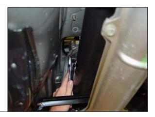
STEP 11. Remove shifter from car. (metal plate and spring will be used on new shifter)
