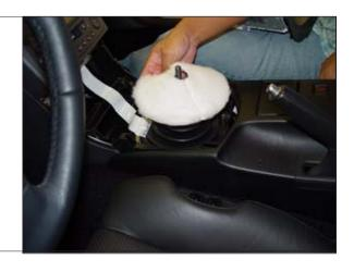
**STEP 5.** Remove shifter cover bolts and wire harness connections, then remove plate from vehicle.
