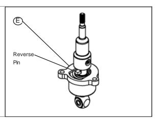
STEP 16. Install stock spring and shifter using stock plate and M6 bolts, washers, then serrated washers Make sure that reverse pin is turned towards passenger side of vehicle. TOOLS: Socket Drive, Extension, and Hex Drive(5 mm)
