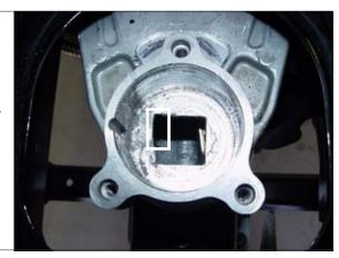
STEP 13. If you were unable to remove the shift knob in step 1, then carefully place the knob in a vise (shifter inverted) and using the long extension or other long tool through the lower connection hole, carefully rotate (unscrew) the shifter assembly off of the shift knob.
