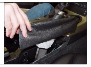
**STEP 15.** Remove (2) bolts holding down front center console. TOOLS: Ratchet, Extension & Socket (7mm)
