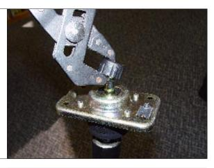
STEP 22. Install plastic pivot cup onto bottom of B&M shifter.
