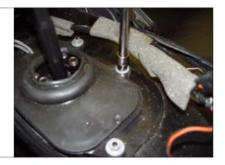
STEP 20. Remove (4) bolts securing shifter and remove from vehicle. NOTE: Shifter shown out of car for clarity only.
