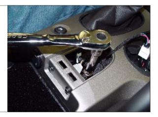
STEP 12. Remove (4) bolts securing arm rest and remove arm rest. TOOLS: Ratchet, Extension & T-15
