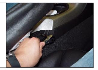
**STEP 16.** Remove passenger side panel and lift up on front center console.
