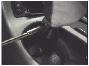
STEP 19. Remove foam and (4) nuts securing rubber. TOOLS:Ratchet, Extension & Socket (10mm)
