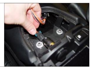
**STEP 44.** Reinstall traction control panel and connect all wires. TOOL: Small Flatblade Screwdriver
