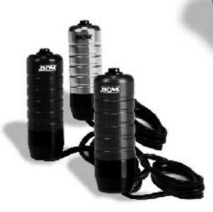
These Hi-tech **Button Knobs** can be used to control any 12-volt function in your vehicle. They feature a momentary switch in a billet aluminum anodized knob. Suitable for nitrous or line lock systems. Fits metric thread sizes: M16x1.5, M12x1.75, M12x1.25, M10x1.5 and M10x1.25 shifter sticks. Knob measures 3.75" in height.
