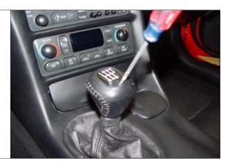
**STEP 2.** Remove small metal insert. TOOL: Vise grips
