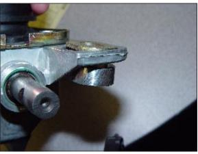
**STEP 26.** Install bolts securing shifter base to vehicle. TOOLS: Ratchet, Extension & T-40
