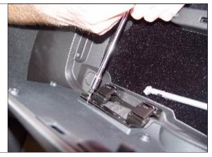
STEP 13. Remove (2) screws under passenger airbag panel. TOOLS: Ratchet, Extension & Socket (7mm)
