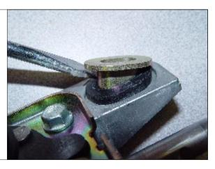
**STEP 25.** Install bushing underneath housing as shown.
