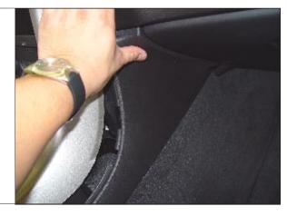
**STEP 33.** Reinstall (2) bolts holding down front center console. TOOLS: Ratchet, Extension & Socket (7mm)
