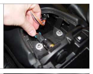
STEP 6. Remove panel next to ignition key (temperature sensor) and remove screw. TOOLS: Small Flatblade Screwdriver, Ratchet, Extension & T-15
