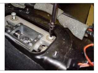
STEP 24. Remove stock rubber bushings. TOOL: Small Flatblade Screwdriver
