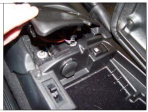
**STEP 5.** Remove (2) retaining nuts and wire connectors. TOOLS: Socket(10 mm), Drive, and Extension.
