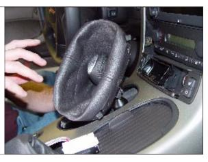
**STEP 18.** Remove screw securing knob and lift out front center console. Be sure to remove connector wires. TOOL: Ratchet, Extension & T-20
