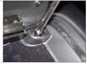
**STEP 9.** Slide rear center console back enough to remove front center console. Remove front center console.
