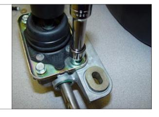
STEP 21. Remove pivot cup from bottom of stock shifter. TOOLS: Channel Locks
