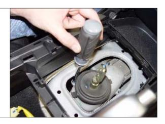
STEP 10. Remove bolts (4) and screws (3) holding down shifter.
