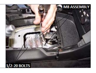
Torque 1/4-20 bolts to 8-10 ft-lbs. Caution do not overtorque bolts!! Torque M8 thin nuts to 8-10 ft-lbs. Torque M8 nuts to 15 ft-lbs.
