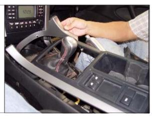
STEP 25. Reinstall screw for console. TOOLS: Screwdriver (phillips)
