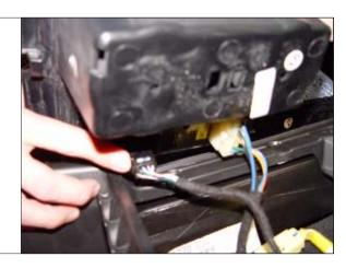
**STEP 3.** Pull up and remove center console.
