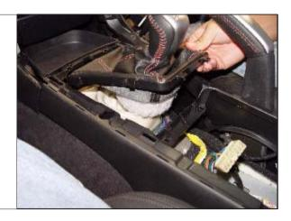
**STEP 21.** Reinstall wires onto windows and T/C switches on center console.
