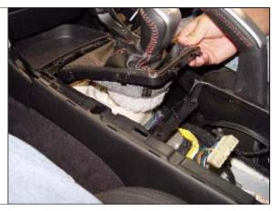
**STEP 5.** Remove bolts (2) securing top stick of stock shifter. TOOLS: 10mm socket & Drive.
