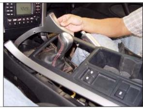
STEP 4. Pull up on plastic retainer for shift boot.
