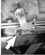
B. Gradually tighten the cable nuts against the bracket while continuing to check the fit of the swivel in hole "F" in the selector lever. Then with the swivel inserted in the selector lever, lightly snug the jam nut.
