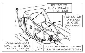
10. Route the cable approximately as shown, based on your application. Avoid any sharp bends which may kink or otherwise damage the cable. Seal the cable hole shut to keep exhaust fumes, water, etc. out of the passenger
