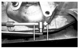
**16.** Thread the swivel onto the cable to about the middle of the threaded section, then reinstall (but do not tighten) the jam nut.
