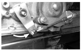
**37.** With the swivel still in the selector lever, operate the shifter through each position, verifying that the swivel slips freely in and out of the lever in each position.
