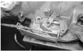
15. Attach the shifter cable to the cable bracket: First remove the small jam nut, two plastic dust boots, and one large nut and lock washer from the cable. Then insert the cable through the cable bracket, reinstall the lock washer and nut on the cable (loosely, to allow room for adjustment), and reinstall the two dust boots.
