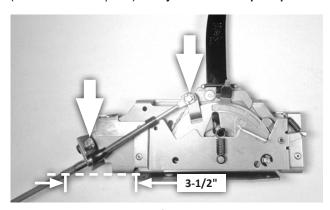
7. Assemble the cable and shifter. Secure the cable eye to the shifter pin with a 1/4" I.D. e-clip. Then secure the cable's mount tab to the outside surface of the shifter base with the 1/4-20 × 1/2" bolt and a 1/4" nut (apply medium strength thread-locking fluid to the bolt).
