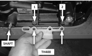
**46.** Check cable bracket fit: Remove the two oil pan bolts to the rear of the selector shaft. Determine which cable bracket holes will be used on your transmission.
