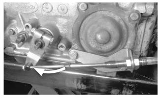
**36.** With the swivel still in the selector lever, move the shifter to the PARK (full-forward) position. Verify that the swivel still slips freely in and out of the selector lever. If not, adjust the large cable nuts (and the swivel, if necessary) until it does.
