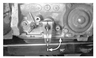
**30.** Install the B&M selector lever using the 1/4-20 × 1-1/2" bolt, and a 1/4" lock washer and nut. With the selector shaft in NEUTRAL (the second click back from PARK, which is full-forward), align the selector lever perpendicular to the oil pan split-line, then tighten the fasteners.
