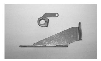
**11.** Get the Chrysler / AMC selector lever and cable bracket from the parts kit.
