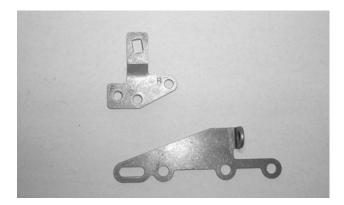
**43. Get the GM selector lever and cable bracket** from the parts kit.
