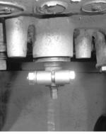
**NOTE:** If the selector shaft is grooved as shown, center the lever between the groove and the end of the shaft, so that the lever's inboard clamping surface does not land in the groove.
