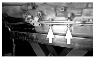
A. For stamped sheet-metal (stock) pans, use the two spacers between the pan and bracket.
