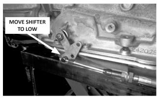
**54.** With the swivel still in the selector lever, ratchet the shifter back to your transmission's lowest gear (for 3-speeds), or to its second-lowest gear (for 4-speeds; see NOTE below), verifying that the swivel slips freely in and out of the lever in each position.
