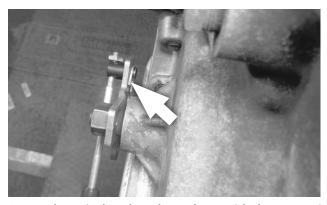
**55.** Secure the swivel to the selector lever with the cotter pin. Operate the shifter through all the gear positions, verifying that it operates correctly.
