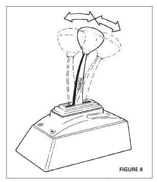
To shift the transmission in Ratchet Shift mode, simply pull or push the shift lever to a full stop then release it, allowing it to return to its "centered" position (Figure 4). Repeat this action until the transmission is in the desired gear.
