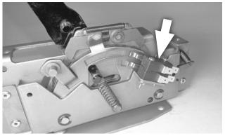
Install the two micro-switches on the shifter mechanism as shown, using the two #4-40 × 1-1/4" screws, lock washers and nuts.
