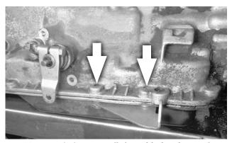
6. C6 transmissions: Install the cable bracket at the two left rear oil pan bolt holes, using the two 5/16-18 × 1" bolts and flat washers. For stamped sheet-metal (stock) pans, use the two spacers between the pan and bracket. (Spacers are not used with cast aluminum pans.) Tighten the bolts to 12-13 ft-lbs torque.
