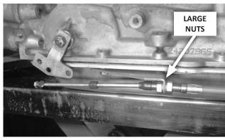
**48.** Attach the shifter cable to the cable bracket: First remove the small jam nut, two plastic dust boots, and one large nut and lock washer from the cable. Then insert the cable through the cable bracket, reinstall the lock washer and nut on the cable (loosely, to allow room for adjustment), and reinstall the two dust boots.
