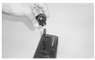
**67. Apply medium strength thread locker** to the shift lever threads. Carefully thread the **shift knob** all the way onto the lever and hand-tighten.
