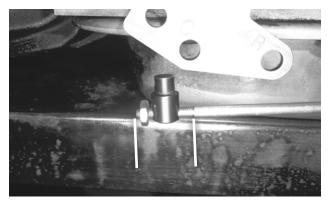
**49.** Thread the swivel onto the cable to about the middle of the threaded section, then reinstall (but do not tighten) the jam nut.
