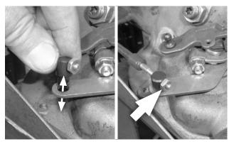
18. When the swivel slips freely in and out of the selector lever, snug the jam nut.
