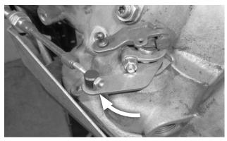
**20.** With the swivel still in the selector lever, operate the shifter through each position, verifying that the swivel slips freely in and out of the lever in each position.
