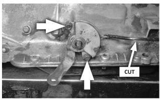
28. If your transmission is equipped with a neutral safety / backup light switch: Remove the two mount bolts and slide the switch off the selector shaft. Cut the wiring harness between the switch and its connector, and discard the switch. (The wires from the connector will be routed to the B&M switches later.)
