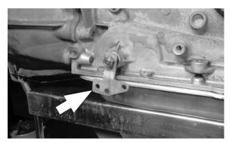
**45. Install the B&M selector lever** using the stock selector lever nut, and tighten the nut to 23 ft-lbs torque. The lever should travel smoothly back and forth, with a positive "click" in each detent.
