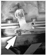
**52.** When the swivel slips freely in and out of the selector lever, snug the jam nut.
