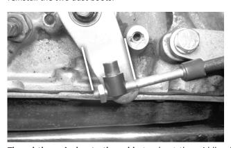
**33.** Thread the swivel onto the cable to about the middle of the threaded section, then reinstall (but do not tighten) the jam nut.
