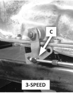
51. Adjust the large cable nuts until the swivel slides freely in and out of the correct hole in the selector lever (hole F for 4-speeds; hole C for 3-speeds). Gradually tighten the nuts against the cable bracket, while continuing to check the fit of the swivel in the selector lever.
