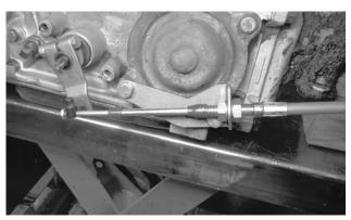
**32.** Attach the shifter cable to the cable bracket: First remove the small jam nut, two plastic dust boots, and one large nut and lock washer from the cable. Then insert the cable through the cable bracket, reinstall the lock washer and nut on the cable (loosely, to allow room for adjustment), and reinstall the two dust boots.
