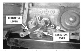
**27. Disconnect stock controls:** Remove and retain the nut and lock washer holding the throttle lever on its shaft. Carefully remove the throttle lever, and move it and its linkage aside, allowing them to hang free. Remove and discard the stock shift linkage.
