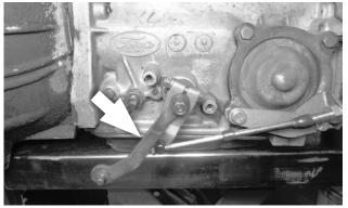
**39. Reinstall the throttle lever, lock washer and nut** on the throttle shaft and tighten securely. The throttle lever must operate smoothly with no binding.
