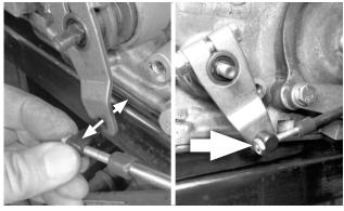
35. When the swivel slips freely in and out of the selector lever, snug the jam nut.
