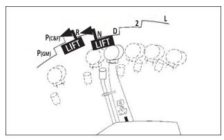
The lockout trigger must be lifted to move:
