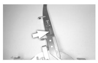
**57. Install the red position indicator tape** on the left side of the shift lever, as shown — just below the rear leg of the letter "M," and parallel to the rear edge of the lever.
