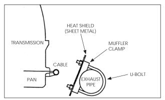
**CAUTION:** Heat will severely damage the shift cable, causing the housing to melt or become brittle. If the cable must be routed near exhaust system components, fabricate a heat shield. **Do not wrap the cable, as this retains heat.**
