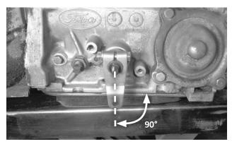
28. Install the B&M selector lever using the 1/4-20 × 1-1/2" bolt, lock washer and nut. (See NOTE on next page.) With the selector shaft still in NEUTRAL, align the selector lever perpendicular to the oil pan split-line, then tighten the fasteners.
