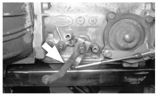
35. Reinstall the throttle lever, lock washer and nut on the throttle shaft and tighten securely. The throttle lever must operate smoothly with no binding.
