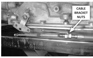
44. Attach the shifter cable to the cable bracket: First remove the small jam nut, both plastic dust boots, and one large nut and lock washer, from the cable. Then insert the cable through the cable bracket, reinstall the lock washer and nut (loosely, to allow room for adjustment), and reinstall the dust boots.
