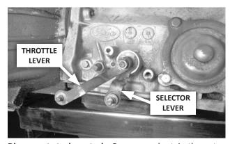
**25. Disconnect stock controls:** Remove and retain the nut and lock washer holding the throttle lever on its shaft. Carefully remove the throttle lever, and move it and its linkage aside, allowing them to hang free. Remove and discard the stock shift linkage.
