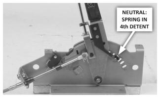
With the selector lever still in NEUTRAL (2 clicks from PARK) and the shifter in the NEUTRAL position (shown), adjust the cable bracket nuts (and swivel, if necessary) until the swivel slips freely in and out of the selector lever hole.
