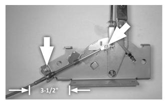
8. Assemble the cable and shifter. Secure the cable eye to the shifter pin with the 3/32" (large diameter) cotter pin. Then secure the cable's mount tab to the outside surface of the shifter base with the 1/4-20 × 1/2" bolt and nut (apply medium strength thread-locking fluid to the bolt).
