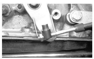
**31.** Thread the swivel onto the cable to about the middle of the threaded section, then reinstall (but do not yet tighten) the jam nut.
