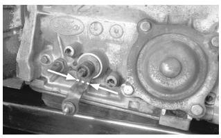
**27.** Move the selector lever to NEUTRAL (2 clicks from PARK). If the selector lever points downward, cut it off at the inboard bend, to allow correct positioning of the B&M lever.
