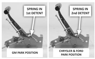
CAUTION: The shifter has two PARK positions — the first (lever full-forward) is for GM transmissions; and the second (one position back) is for Chryslers and Fords. Once shifter installation is completed, always push the lever FULLY FORWARD to put the transmission into PARK. Otherwise the transmission's park pawl will not engage, which will allow the vehicle to roll.
