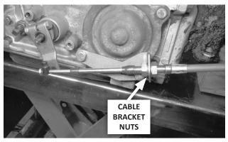
**30.** Attach the shifter cable to the cable bracket: First remove the small jam nut, both plastic dust boots, and one large nut and lock washer, from the cable. Then insert the cable through the cable bracket, reinstall the lock washer and nut (loosely, to allow room for adjustment), and reinstall the dust boots.
