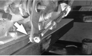
34. Secure the swivel to the selector lever with the 1/16" (small-diameter) cotter pin. Operate the shifter through all the gear positions, verifying that it operates correctly.
