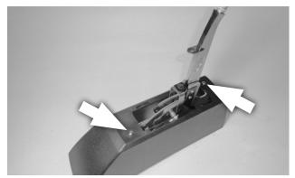
**56.** Once the tower is trimmed to fit, verify the shifter mechanism is free of any debris and loose hardware. Then install the tower using the two #10 self-tapping screws.
