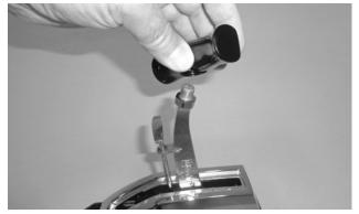
**61. Carefully thread the jam nut** all the way onto the stick, followed by the T-handle.
