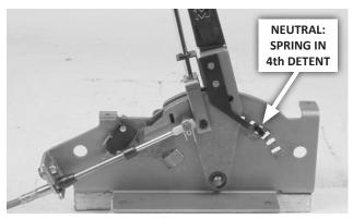
A. Manually move the selector lever to the NEUTRAL detent (2 clicks back from full-forward), and move the shifter to the NEUTRAL position. Adjust cable bracket nuts (and the swivel, if necessary) until the swivel slips freely in and out of the selector lever hole.
