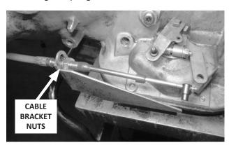
**15.** Attach the shifter cable to the cable bracket: First remove the small jam nut, both plastic dust boots, and one large nut and lock washer, from the cable. Then insert the cable through the cable bracket, reinstall the lock washer and nut (loosely, to allow room for adjustment), and reinstall the dust boots.
