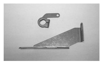
11. Get the Chrysler / AMC selector lever and cable bracket from the parts kit.
