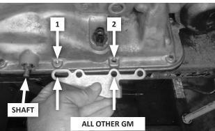
**42.** Check cable bracket fit: Remove the two oil pan bolts to the rear of the selector shaft. Determine which cable bracket holes will be used on your transmission.
