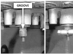
**NOTE:** If the selector shaft is grooved as shown, center the lever between the groove and the end of the shaft, so that the lever's inboard clamping surface does not land in the groove.
