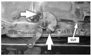
**26.** If your transmission is equipped with a neutral safety / backup light switch: Remove the two mount bolts and slide the switch off the selector shaft. Cut the wiring harness between the switch and its connector, and discard the switch. (The wires from the connector will be routed to the B&M switches later.)
