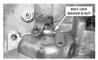
**13.** Install the B&M selector lever using the 1/4-20 × 1-1/2" bolt, and a 1/4" lock washer and nut. Be sure the lever is not pushed down against the transmission case, which could cause binding. The lever should travel smoothly back and forth, with a positive "click" in each detent. Then reinstall the throttle lever and linkage, tighten its pinch bolt securely, and check for smooth operation.
