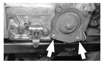
A. <u>C4 / C5 transmissions</u>: Install the cable bracket at the two lower servo cover bolt holes, using the two 5/16-18 × 1" bolts, flat washers and spacers. Tighten the bolts to 12-13 ft-lbs torque.
