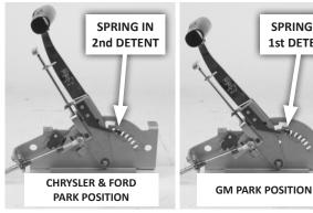
**CAUTION:** The shifter has two PARK positions — the first (lever full-forward) is for GM transmissions; and the second (one position back) is for Chryslers and Fords. To avoid stretching the shifter cable when shifting into PARK, NEVER force the shifter past the second (rear) PARK position (which corresponds to your transmission selector lever's PARK detent).
