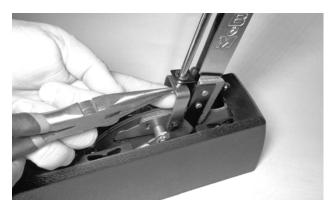
**58. Slip the chrome cover over the shift lever,** but temporarily support it as far upward and rearward as possible. Then reinstall the trigger assembly, the brass washer, and the spring clip.
