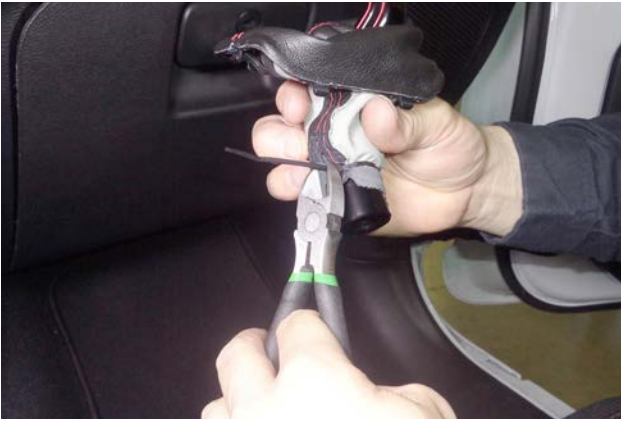
14. Trim the tail off the cable tie.
