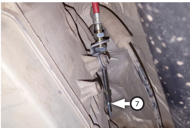
20. Thread locking washer, nut (7) , cable cap and remaining nut onto cable as shown.
