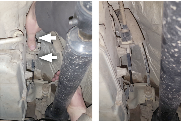
13. Remove (x2 ea.) bolts securing shifter cable to transmission.
