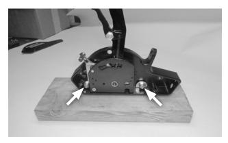
2. Remove the 2 mount screws and nuts.
