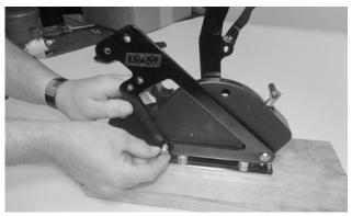
3. Assemble the bracket to the right side of the shifter using the two 5/16" screws against the bracket, and the two 5/16" washers and nuts inside the shifter. (Use anti-seize compound to prevent galling.)
