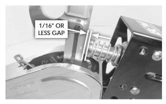
**10.** Move the shift lever to SECOND gear. While holding the solenoid plunger, adjust the nut on the back of the solenoid until there is a visible gap not greater than 1/16" between the plunger and the lever.
