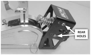
B. Use the rear holes with 3-speed transmissions.
