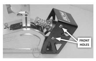
A. Use the front holes with 2-speed transmissions.
