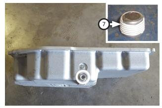
9. Apply Teflon tape to **socket plug (7)** before installing it into deep pan.
