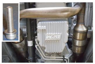
Use lint free rag to clean transmission pan mounting surface, then install deep pan with (x15 ea.) screws (2) and flat washers (3). Torque screws to 8 ft/lbs.
