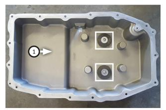
7. Install (x2) screws (5) through (x2 ea.) lock washers (4), flat washers (6), and magnetic rings (9) then into deep pan (1).
