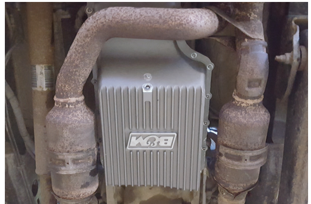
13. Fasten transmission gasket and pan in place using (x19 ea.) screws (4) and washers (5) .
