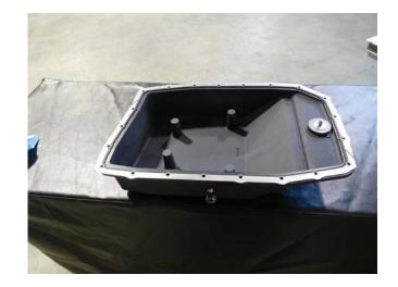
5. Clean the transmission mounting surface and install the B&M pan onto the transmission with the supplied M6 allen bolts and washers, qty. 21. Torque pan bolts to factory torque specs. Then follow your stock re-fill procedure. NOTE: Make sure transmission filter is pushed up into place inside the transmission.
