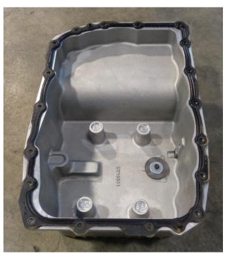
6. Clean the transmission mounting surface and install the B&M pan onto the transmission with the supplied M6 allen bolts and washers, qty. 18. Torque pan bolts to factory torque specs.
