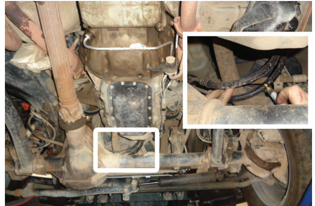
14. Identify and mark factory transmission return line.
