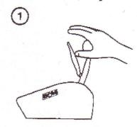
1st gear ready position. Hand off trigger, stick all the way back.
