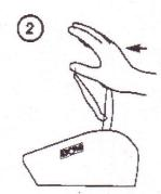
1-2 shift. Hand off trigger, slap knob forward to 2nd gear locked position.
