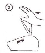
1-2 shift. Hand off trigger, slap knob forward to 2nd gear locked position.
