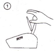
1st gear ready position. Hand off trigger, stick all the way back.
