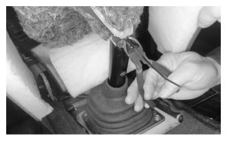
**28. Secure the boot to the lever** with the new cable tie, locating the buckle at the flat at the rear of the groove. Tighten the cable tie, and cut off the tail.
