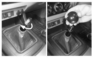
**34.** Run the jam nut all the way down the threads, then install the shift knob
