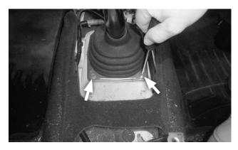
8. Remove the 2 screws at the rear of the cover plate assembly.
