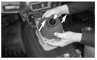
**10. Remove the cover plate,** working the rubber boot up over the shift lever.
