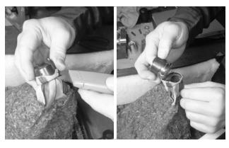
**26.** On the upper console panel, turn the leather boot insideout, carefully cut and remove the tie-off string, and remove the chrome trim ring.
