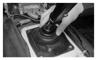
**22. Install the lower dust boot over the shift lever,** and work it down over the rubber boot on the shifter.
