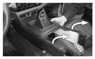
**7.** Remove the front console by first lifting its rear end, then moving the whole console rearward.
