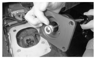
**16.** On the B&M shifter, lubricate the pivot bushing o-rings, and align the bushing with the lever centerline (make sure it's not cocked).
