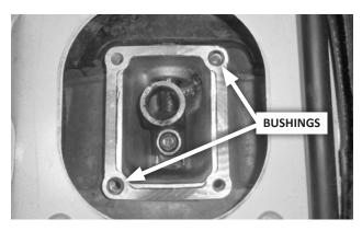
**13.** If either of the 2 alignment bushings remains with the shifter, return them to their locations on the shifter mount pad.
