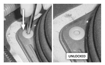
9. Unlock the 2 plastic push rivets at the front of the cover plate by depressing their center plungers slightly (about 1/16") with a punch or small Phillips head screwdriver.
