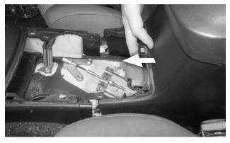
**30. Slide the rear console forward,** engaging both the 2 top tabs, and the 4 locking tabs (2 on each side), with the front console.
