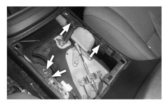
31. Reinstall the 4 forward screws.
