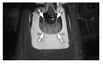
11. Put the shifter in NEUTRAL, then remove the 4 mount screws.
