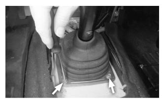
25. Re-install the 2 cover plate screws.
