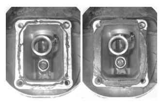
**15.** Apply a thin bead of oil resistant RTV silicone gasket maker to the shifter mount pad, then spread it over the mating surface.
