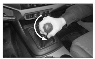
1. Remove the shift knob by unscrewing it from the shift lever.
