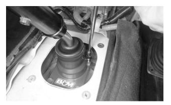
**18. Re-install the 4 stock shifter screws,** and tighten to 15 ft-lbs torque.
