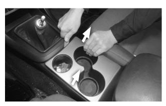
**2. Use a plastic trim removal tool** to separate and remove the cup holder from the console.
