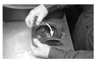
**21.** Carefully peel the lower dust boot off of the cover plate assembly.
