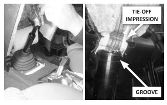
**27. Move the shift lever into 4th gear.** With the leather boot still turned inside-out, work its opening down over the shift lever until the impression from the tie-off string is located over the groove on the lever.
