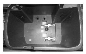
**32. Reinstall the 2 storage compartment screws** and reinstall the felt liner.
