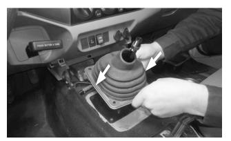
**23.** Lower the rest of the cover plate assembly over the shift lever, carefully working the boot's opening around the screw heads on the lever.
