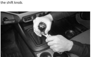
**35. Turn the knob all the way down** until it touches the nut. Then back it off to align it as desired, and tighten the jam nut.
