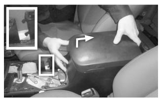
**6. Lift the rear console slightly** and move it slightly rearward to separate it from the front console. (Note the two locking tabs on each side.)
