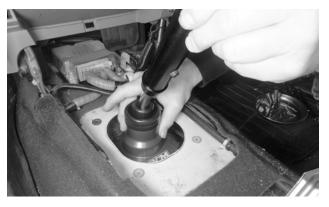
**17. Install the shifter on the mount pad.** First insert the pivot bushing into the shift linkage. Then align the 2 mount pad bushings.
