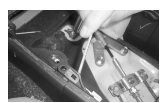
With a small flat-tip screwdriver, separate the 2 tabs from their pins at the joint between the front and rear consoles (1 tab on each side).
