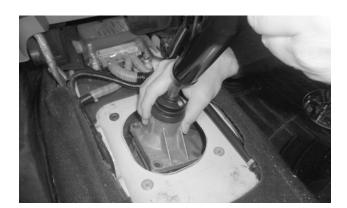
**12.** Remove the shifter from the transmission as follows: Grasp the shifter housing and lever together, as a unit, and carefully tilt them off the mount pad, so as to break the adhesion of the RTV sealant between the shifter and transmission.
