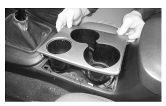
33. Reinstall the cup holder in the console base.
