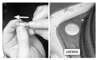
**24. Re-set the plungers on the 2 push rivets** by pushing them up from the bottom end. Then insert the fasteners in their holes and lock them by pushing the plungers down flush.
