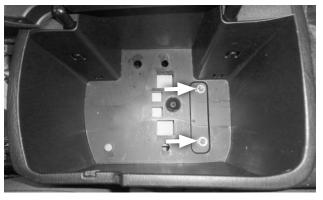
**4. Open the console storage door,** remove the felt liner, and remove the 2 screws.
