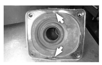
**20. On the cover plate assembly, remove the 2 staples** that hold the upper and lower dust boots together.
