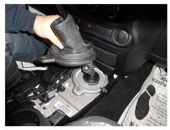
4) Use a ratchet and T45 torx socket to remove the bolt in the center of the shifter.
