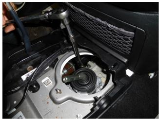
15) Reinstall the shifter donut from the interior side down over the shifter.
