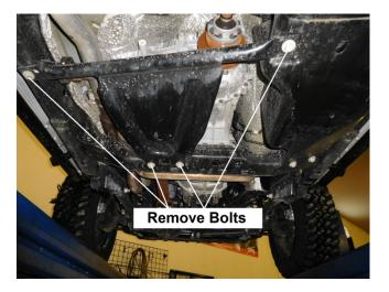
6) Use a ratchet and 18mm socket to remove the 4 bolts securing the transfer case skid plate.
