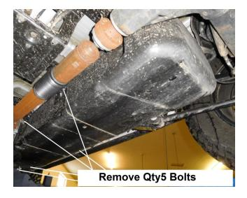
8) Support the center of the transmission crossmember with a jack or a stand. Remove qty. 4 bolts to lower the transmission down roughly 2"- 4".
