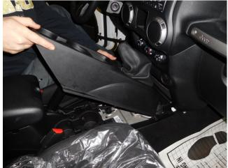
3) Unscrew the square secure plate holding the rubber boot over the shifter. Then remove the rubber boot.
