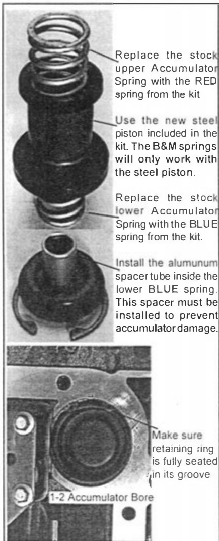
Figure 6. 1-2 Accumulator assembly
