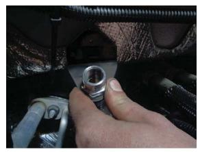
Arrange tube so there are no kinks along its length then set mount on firewall. Repeatedly remove and insert dipstick into tube to ensure it wont bind once tube is secured.
