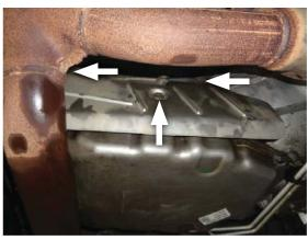
14. Install bolts (x3) to fasten cover (removed step 5) to passenger side of transmission.
