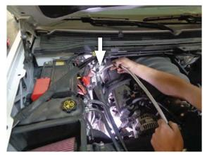
7. Place tube (1601021) into vehicle near engine firewall.
