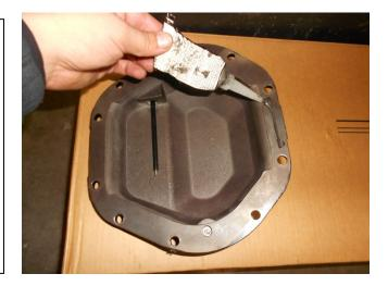
10. Install the B&M Cast Iron Rear Diff Cover on the axle housing using the supplied qty10 5/16" bolts and washers.
