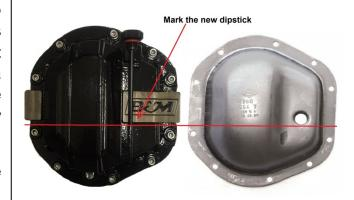
9. Apply a bead of RTV silicone gasket maker to the B&M Cast Iron Diff Cover. Run the bead inside the bolt holes. If your vehicle has a reusable gasket it may be reused but check the condition of it.
