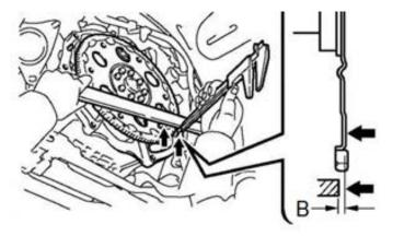
B. Measure Dimension B: On the engine, measure the distance between the engine block mating surface and the torque converter mating pads (the raised surfaces on the flexplate at each torque converter fastener hole).
