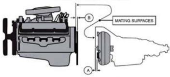
C. Verify that Dimension A is greater than Dimension B. If it is not, the torque converter is not fully seated. Pull it off slightly, then, while rotating it, push it back on. Continue to do this until you feel the torque converter move inward and make the proper engagement. Then repeat and compare Dimensions A and B. Do not proceed further until the torque converter is fully seated.
