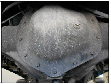
8. Using a razor blade or gasket scraper, clean all gasket material from the axle housing surface (See Figure 2).
