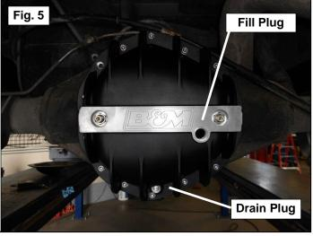
18. Install the axle housing fill plug and torque to 20ft/lbs.
