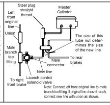
BRAKE AND THE LEFT REAR BRAKE ARE ON ONE CIRCUIT WITH THE LEFT FRONT BRAKE AND RIGHT REAR BRAKE ARE ON THE SECOND CIRCUIT. FOR SYSTEMS, THESE IS IΤ RECOMMENDED THAT TWO LAUNCH CONTROLS BE UTILIZED ONE IN EACH SYSTEM. Illustrations are given for the hydraulic portion of six typical single and dual master cylinder brake systems. These represent the hydraulic system of most domestic and import vehicles. The electrical section of the
