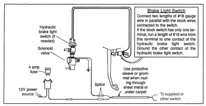
insulated connector. All soldered connections should be wrapped with plastic electrical tape. All wires should be as short and direct as possible, but not short enough to put any tension on the wires. Electrical wires should not be under tension even when the engine and transmission move on the their mounts.
