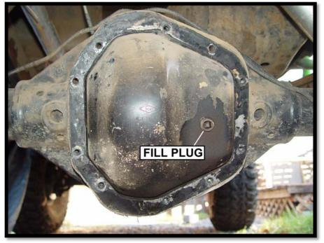
vehicle 1-2 feet so you will have plenty of room to work. Also, have a small box to put bolts in and a drain pan to catch oil.
