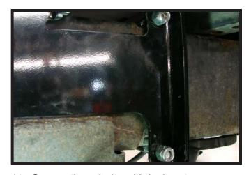
11. Secure the u-bolts with lock-nuts.
