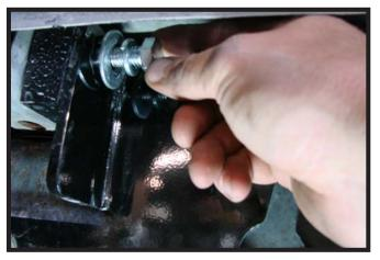
9. Install both side plates and insert corresponding hardware.
