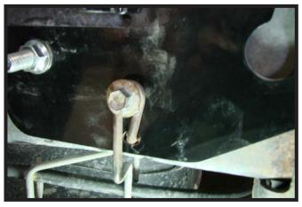
13. Reinstall emergency brake line bracket using the existing bolt through the two hole in the side plate.
