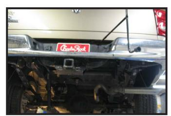
Using the vehicles jack handle tool, remove the spare tire as per vehicles owners manual.
