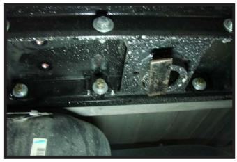
8. Install the center section in between the cross-members and up through the 5" hole in the truck bed. Insert all bolts into the cross-members and center section.
