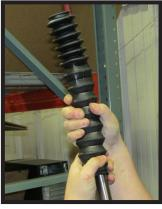
3. Coat the inside of the new boot with silicone spray, clean and re-grease the leg assembly, and install the new boot.
