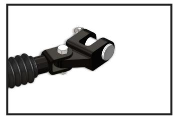
Install the offset double lug onto the tow bar leg with the new washers, 1/2"-13 x 2" bolt and 1/2"-13 jam nut provided. Tighten the bolt until the lug is tight against the washers, but can still freely move side to side. Do this on both tow bar legs.
