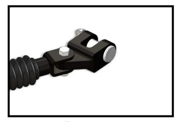
Install the offset double lug onto the tow bar leg with the new washers, 1/2"-13 x 2" bolt and 1/2"-13 jam nut provided. Tighten the bolt until the lug is tight against the washers, but can still freely move side to side. Do this on both tow bar legs.
