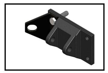
3. **Optional Safety Cable Bracket:** Remove the two (2) inside existing bolts from the bumper d-link bracket. Install the safety cable bracket onto the d-link bracket with the 12MM x 50MM bolts and 12MM hex nuts supplied. Do this on both sides of the vehicle.
