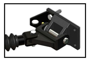
Install the tow bar onto the bumper d-link brackets with the 5/8" pin and lynch pin. Using the plastic spacers as required in between the lug and d-link as shown.
