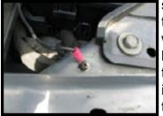
screw. Locate this screw on the inner fender area close to the fuse panel so that when installed there is sufficient wire to lay the Fuse ByPass Switch in a convenient location near the fuse panel. An alternative is to loosen the large ground stud to the left of the fuse box and fully insert the terminal under the ring as shown in the photo, t
