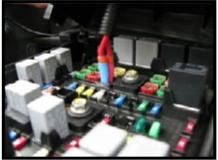
under hood fuse box. Remove the large plastic fuse box cover and remove the high amperage (e.g. 50 amp) fuse. Confirm that the colored connectors on the Fuse ByPass
