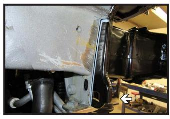
14. Temporarily reinstall the metal bumper.
