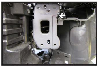
13. Using a reciprocating saw, cut the frame face back to the frame rail then vertically flush with the side of the frame rail all the way down. Do this on both sides of the vehicle.
