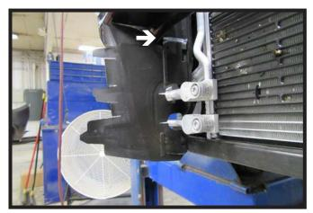
15. Trim the plastic shrouding off just below the bumper. Do this on both sides of the vehicle.
