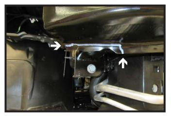
16. Trim the lower lip of the bumper flush with the bumper back approximately 4" from the end for baseplate clearance. Do this on both sides of the bumper.
