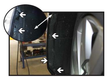
4. Using a T25 Torx, remove the five (5) screws from the edge of the wheel well. Do this on both sides of the vehicle.
