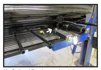
23. **Optional Breakaway:** Attach the breakaway to the baseplate with supplied 1/4"hardware.
