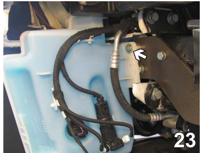
23. Using a 6MM hex bolt lock and flat washer. Install the six 3/8" lock washers between the reservoir and baseplate, then tighten water reservoir to its original location.
