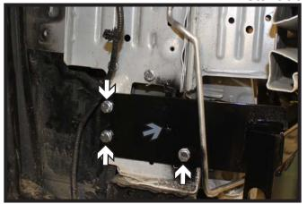
10. Using a 3/8" drill bit, drill the remaining holes in the sideplates thru the frame. Install the 3/8" hardware into the holes. Do this on both sides of the vehicle. Fully tighten all hardware.
