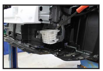
2. **tC models only:** On the driver side, remove the plastic reinforcement and set aside. The reinforcement will not be reinstalled.
