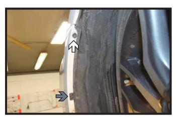
3. Using a 10MM socket, remove the screw from the edge of the wheel well (white). Then turn the locking pin (gray) to release the fascia from the wheel well liner. Do this on both sides of the vehicle.
