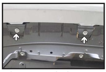
4. Using a 10MM socket, remove the eight (8) screws from the underside of the fascia. There are two (2) on each side and four (4) along the front.
