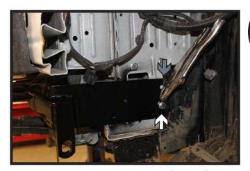
8. Install the baseplate onto the frame, flushing the edge of the sideplate with the frame (gray) and clamp in position. Using a 3/8" drill bit, drill the lower back hole (white) thru the frame. Install the 3/8" hardware into the hole. Do this on both sides of the vehicle. Fully tighten all hardware.
