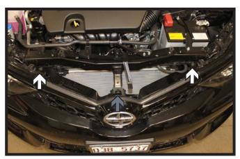
Remove the two (2) push pins from the fascia (white). Then, using a 10MM socket, remove the screw from the center of the fascia (gray).
