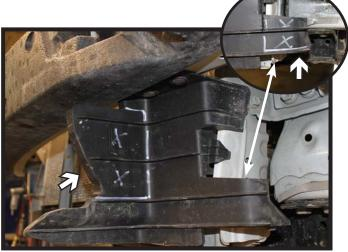
tC models only: On the driver side, trim the plastic shielding under the bumper and towards the outer edge as shown for baseplate clearance.
