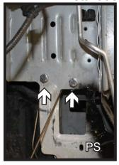
6. Prior to baseplate installation, using a 3/8" drill bit, drill holes in the approximate locations shown on both the driver and passenger sides. Install the 3/8" hardware into the holes and fully tighten all hardware. These bolts will reinforce the frame from delaminating.
