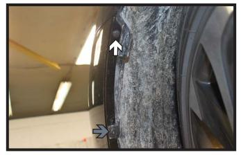
Remove the push pin from the edge of the wheel well (white). Then turn the locking pin (gray) to release the fascia from the wheel well liner. Do this on both sides of the vehicle.
