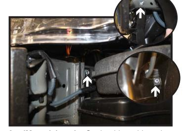
2. **iM models only:** On the driver side, using a 10MM socket, remove the three (3) screws from the baffle. There is one (1) in front under the headlight and two (2) just in front of the wheel well liner (insets). Set the baffle aside.
