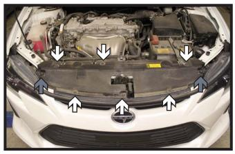
1. Push down on to release and remove the six (6) push pins from the fascia cover (white). Then remove the two (2) bumpers (gray) and set the cover aside.
