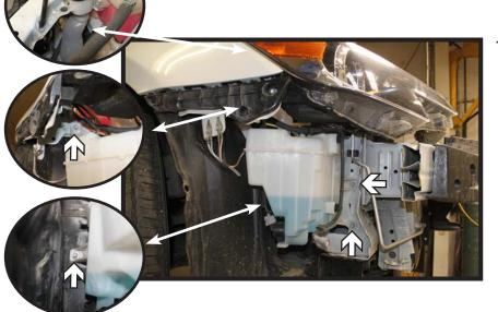
Using a 10MM socket, remove the four (4) screws from the washer reservoir (white). Remove the push pin from the reservoir neck (gray). Disconnect/plug all lines and set the reservoir aside.
