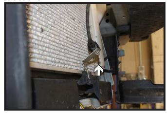
If needed bend the temperature sensor up slightly to allow easier baseplate installation.
