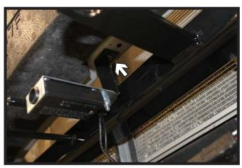
13. **Optional Breakaway:** Attach the bracket to the lip of the bumper at the desired location with the #12 screw provided. Attach the breakaway to the bracket with the 1/4" hardware provided.
