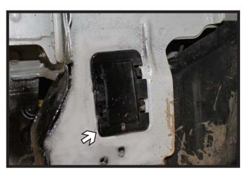
5. **tC models only:** On the driver side, remove the plastic cover along the side of the frame.
