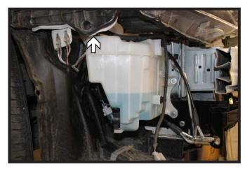
12. Reinstall the washer reservoir with the spacers, 6MM & 1/4" hardware provided. Note: The upper back bolt will not be reinstalled due to the use of the spacers iM models only: Reinstall the baffle on the driver side.
