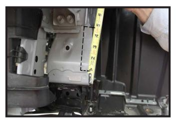
From the bottom of the frame face, measure up 1" & 4-1/2" by 3/4" deep. Using a reciprocating saw, trim a notch in the frame face. Do this to both sides of the vehicle.
