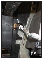
3. **iM models only:** Trim the plastic shielding under the bumper and remove the lower section.
