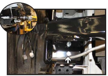
9. Using a 3/8" drill bit, drill the front hole thru the frame. Install the 3/8" hardware into the hole. Do this on both sides of the vehicle. Fully tighten all hardware.
