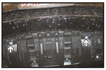
3. Using a 10MM socket, remove the six (6) screws from the underside of the fascia. There are two (2) on each side and four (4) along the front.
