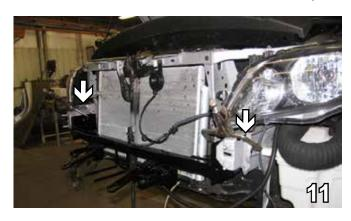
11. Slide the baseplate up between the frame rails, align with the existing hole on each side and clamp.
