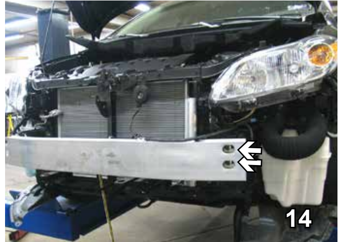
14. Reinstall the bumper. Be sure to reattach the wire loom to the top of the bumper.
